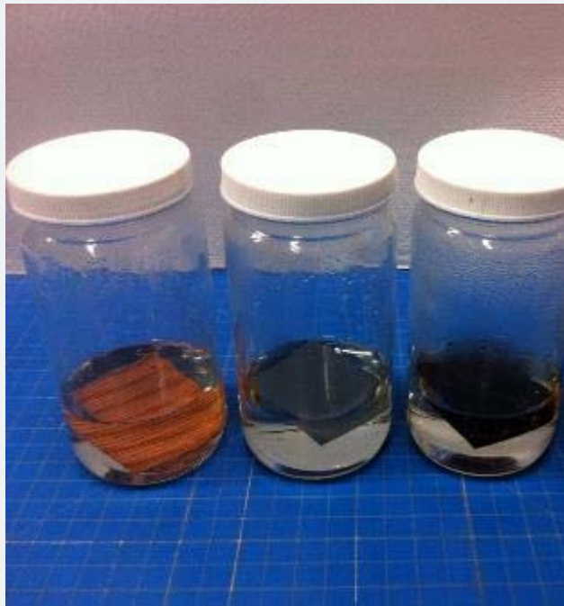
After 20 hrs in H 2 SO 4 at 80 °C
