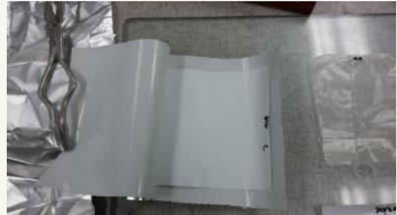
Sealed aluminum pouch for shrinkage testing in electrolyte
